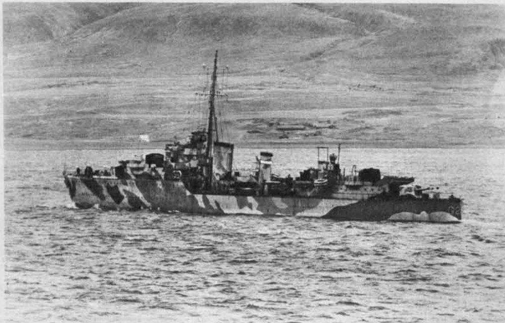
BRITAIN'S TRIBAL CLASS DD's were her answer to the French superdestroyer. They carried eight 4.7-in. guns in superfiring twin mounts forward and aft but only four torpedo tubes.
